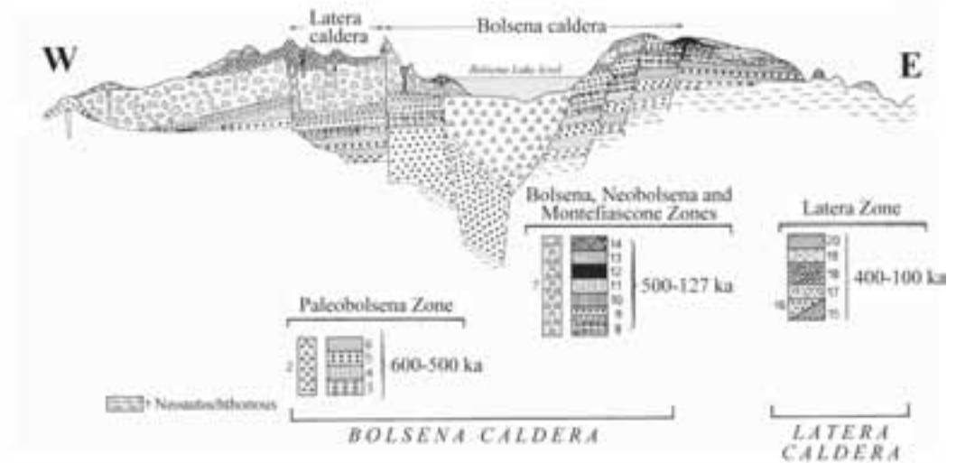
Figure 4 - Space-time evolution of the Vulsini Volcanic Zones visualized through a schematic cross section from W to E of the District (modified from Nappi et al., 1995). Symbols: 1 = clayey-sandy and conglomeratic sediments of marine and brackish environments; 2 = mainly back-fall lithic breccias; 3 = conjectural effusive activity older than the dated plinian pumice falls; 4 = Basal plinian pumice falls; 5 = pyroclastics and lavas; 6 = the Civitella d'Agliano Formation; 7 = mainly back-fall lithic breccias; 8 = pyroclastics and lavas; 9 = Vietena lavic plateau; 10 = Ponticello pumice fall; 11 = Orvieto-Bagnoregio Ignimbrite; 12 = Monterado lava flows; 13 = Montefiascone pyroclastics; 14 = Bisentina Island surtseyan activity; 15 = pre-caldera effusive phase; 16 = Vulci and Monte Calvo lava flows; 17 = ignimbrites; 18 = the Pitigliano Formation; 19 = post-caldera effusive phase; 20 = post-caldera phreatomagmatic eruptions.
